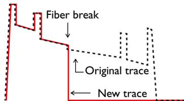
**Note:** An OTDR test can not replace an OLTS measurement. The OLTS test is required by the TIA-standards, and OTDR measurements can slightly under-estimate loss, especially on multimode fibers. An OLTS test would indicate fiber mis-matches of 50/125 and 62.5/125um fibers with a high loss reading. An OTDR which uses a laser and does not fill the outer modes may not pick up the core mismatch.
