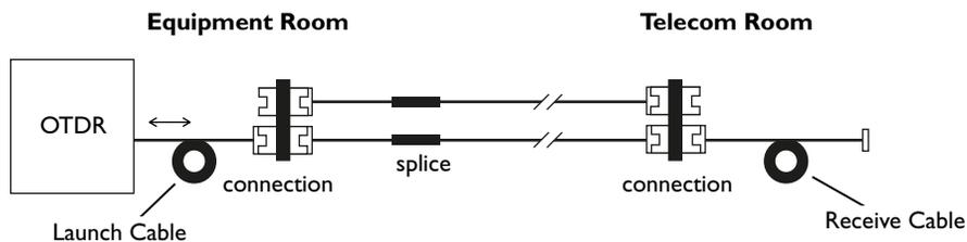
OTDR's operate like a radar. They generate short pulses of light and then sample the light backscattered by fiber segments and related by connections and other events. This allows the user (or OTDR software) to estimate the loss slope or "attenuation" of fiber segments and the insertion loss of individual connections and splices.
