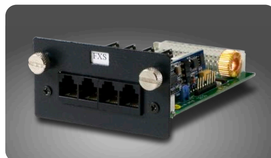
iMux user installable module. Analog POTS module shown.
