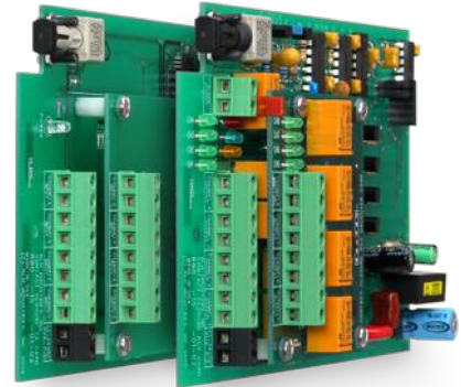
8 Channel Contact Closure Card System
