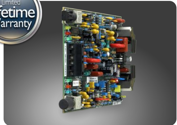
2 Wire Digital Phone Fiber Link Card
