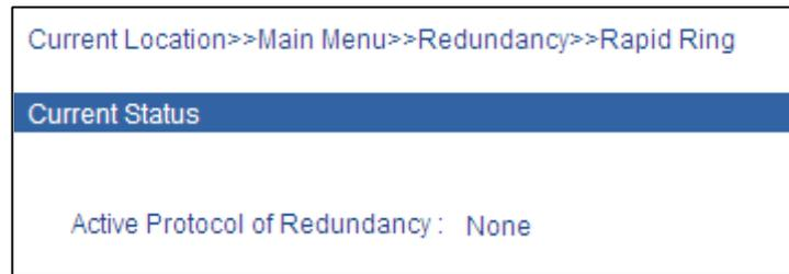
Basic interface shows Protocol of Redundancy is None. Ring can be set by Protocol of Redundancy configuration if it is needed. As shown in the figure below, in [Settings] area there are 2 kinds in corresponding drop-down menu of Protocol of Redundancy: **Ring V2** and **Ring V3**.
