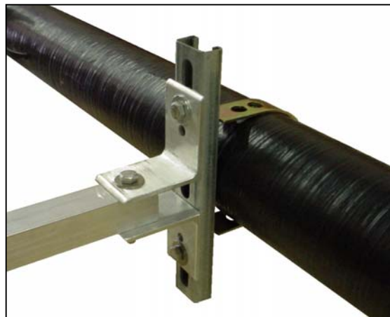
Figure 2 Solar Panel Attachment Slide Nuts Into Lower Channel and Attach Solar Panel Bracket to Channel with Screws and Washers.
