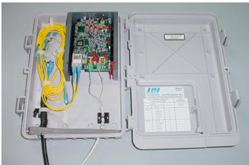
Fig. 4.1 RLH UHDSL CO Card installed inside RLH 2-card indoor/outdoor housing.
