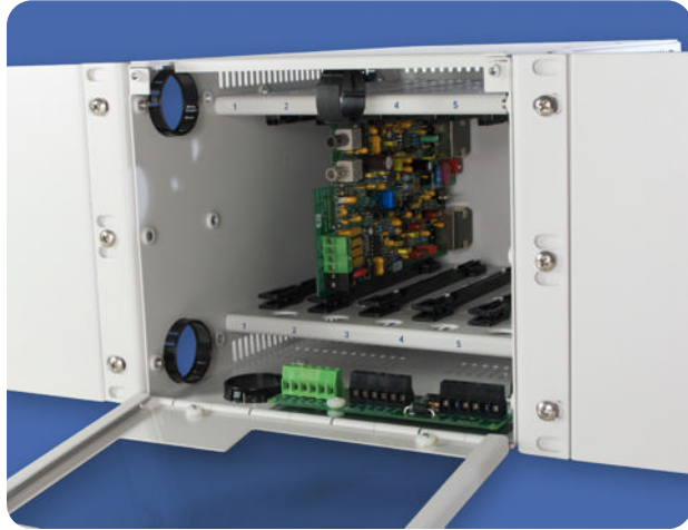
Shown with power terminal and Fiber Optic Link Card installed
