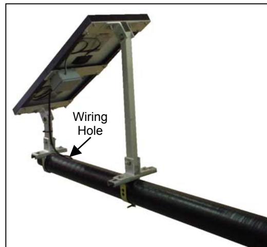
Figure 4 Panel Wiring Insert Solar Panel Wiring Into Hole Located Just Below Top Mounting Bracket and Secure with Ty-Rap's
